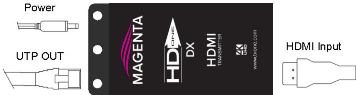
Figure 1 - Connections on the Transmitter
