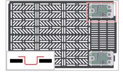
Turn the module over and screw the voltage selector in place with three M4 screws.
