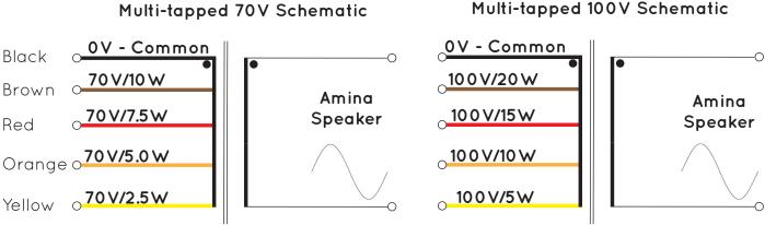
To limit the risk of spurious noise from loose cables, please carefully dress and tie back the unused input taps using a cable tie. See diagram below.
