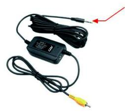
Cut off mini-plug connection of SPS-1 to expose orange, red, and black wires.
