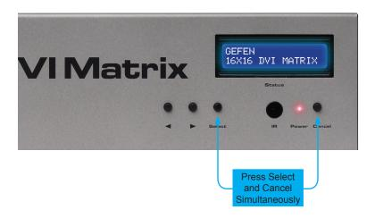
2. The matrix will power-down and go into standby mode.
