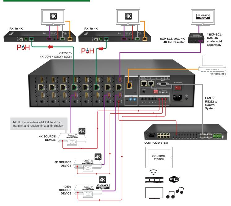
NOTE Serial control at display end requires a compatible model HDBaseT transmission device with routable RS232.
