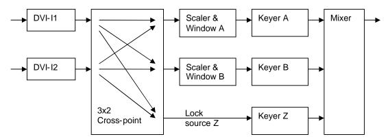
As the diagram shows, the 2 DVI-I inputs are available for use by either of the scalers, or as a 'lock source' (also known as window Z) – where the output is synchronized to an input (see Adjust outputs).
