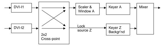
As the diagram shows, the 2 DVI-I inputs are available for use by the scaler, or as a 'lock source' (also known as window Z or background) – where the output is synchronized to an input (see Adjust outputs).
