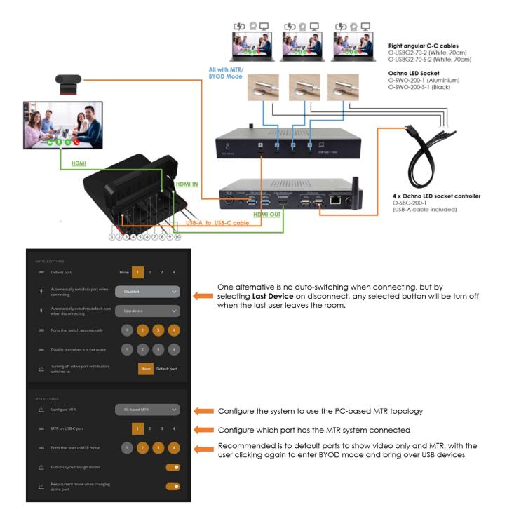
The same considerations in terms of auto-switch or manual switching applies here as for Type B. In the above example there is slight difference in regards to auto-switch from Type B.
