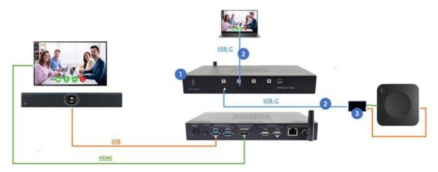
In this setup, the CX-device is active per default, connected via Ochno Power Conference to TV and video conference devices. The CX wireless dongles can be used as usual.
