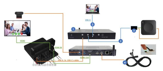
In this setup, both the CX wireless connection and the wired USB-C connection can be used to both run a MTR-hosted meeting or run a meeting from the laptop (BYOD).
