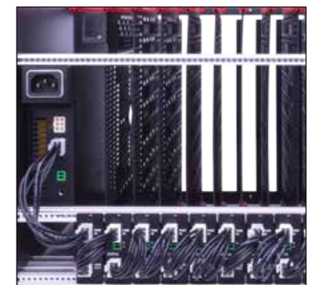
▲ Daisy chaining power eliminate external power supplies and cleans up your racks. Each slot can be set at a different voltage
